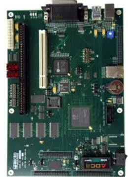
The design is available at no cost and may be used as is or modified to suit specific needs. The [design package](#), available from ZF, includes [OrCad schematic](#), PadsPCB Layout files, and a complete Bill of Materials spreadsheet. Included with the ZFx86 System-On-Chip are a [ZF BIOS](#) (based on Phoenix Technologies kernel), DR-DOS 7.03 license, and software drivers to support all hardware. Additionally, Windows CE® and Linux are available and ready to run.
